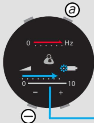
**Power On** - Hold ANY key until power turns on.
